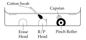
**NOTE:** Never use metal objects on or near the tape heads. Do not allow any cleaning material to fall into the tape assembly.
